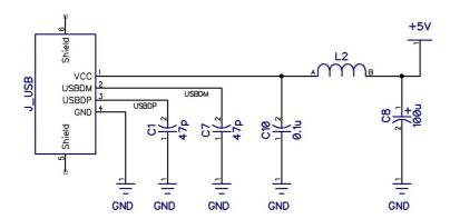
The USB connection has two functions here – it serves as the data link between scope and PC, and in addition it provides the circuit with power.
