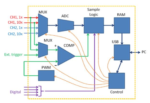
The microcontroller (a Microchip PIC18F14K50) is the heart of the whole instrument. Above you see a high-level block diagram of its internal structure. As said before, almost all functions are integrated into this single chip, Microchip really managed to pack a ton of features into this little marvel costing just around \$3.
