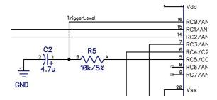
The trigger uses the comparator built into the microcontroller – again great, no external circuitry required for this functionality. The trigger compares the incoming signal (actually the scaled copy of the input signal arriving at the ADC) with a user-controlled threshold level.
