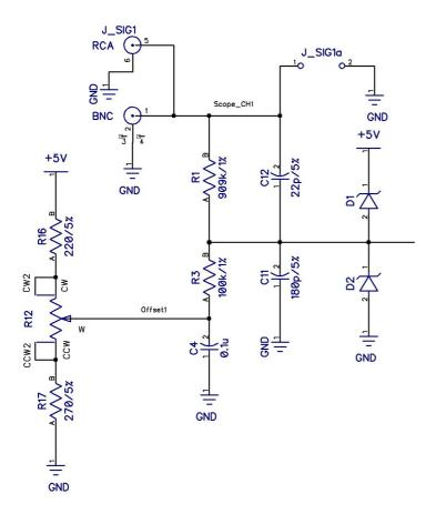
Let's have a look at the input stage first. Since the two channels are identical in their design we will concentrate on scope channel 1 (CH1).
